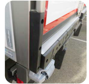
Rear rubber vertical side, protected by sheet metal
