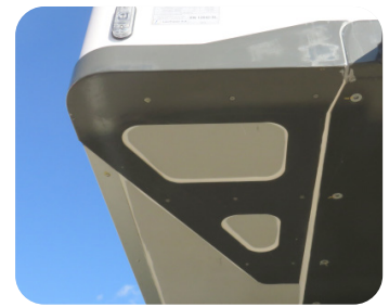
Reinforcement on front corner
