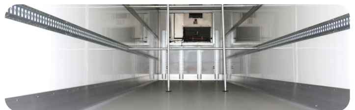
Aluminium floor, aluminium skirting and load-bearing rails
