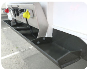
Stainless steel connection bracket, and rubber plate lead up
